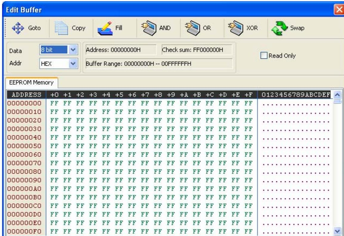
1. Buffer Compile toolbar contains "Set the position of the current cursor" (Position), Copy, Fill, AND/OR/XOR, and exchange between up and low bytes.
