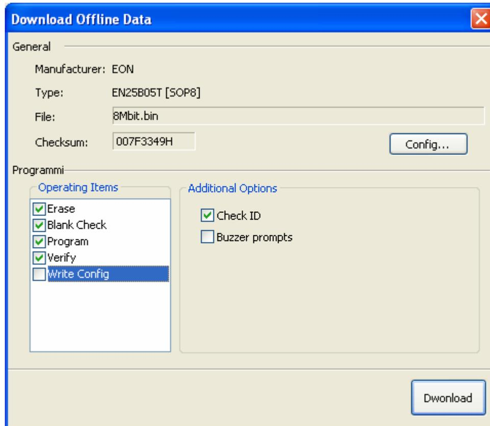
4. Set chip configuration options (Such as, if the current chip doesn't have configuration options, the programmer won't display "Chip configuration").
