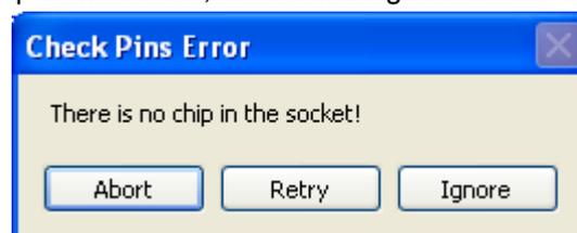
The user can choose to terminate this operation according to his needs, or try again, or skip pin detection and directly go on to program.
